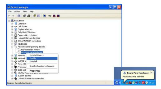
Newer Weather Stations (versions 2.1 and 1.2) include a jumper (pins 9 and 10 for V1.2, and 'AUTO' for V2.1). **If the jumper is OFF (default), the Weather Station will NOT send any data**, so Windows does not assign the "Ballpoint" to this COM, and only when Sportdyno connects to the WS, it will ask for the data. In this way Windows no longer installs the Ballpoint Device.
