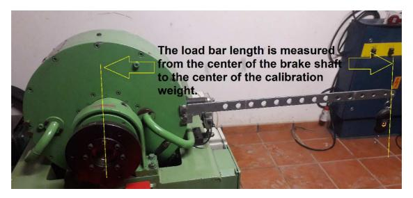
A calibration weight is an important tool, and should therefore be stored and treated as an every important measuring tool.
