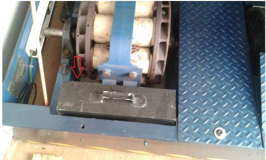
Another example (more critical): the calibration weight must be kept vertical the most balanced as possible. Please note that when the weight leans through front or back the load over the cell will change.
