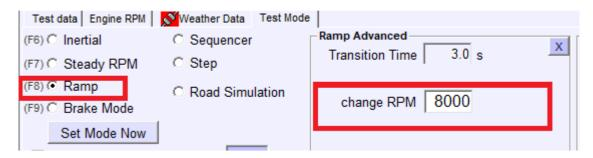
The ramp will start as usual, then will reach the top speed and will start to brake harder while still WOT (Wide Open Throttle). The user should use the clutch to avoid to stall the engine.
