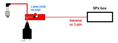
2) TCI Ignition (12V) with **direct connection** for sensing the 300V peaks (the cable is **punctured** to get direct connection)
