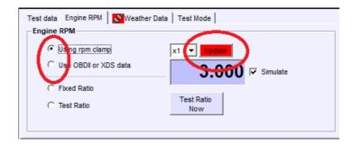
Without OBDII: press the "Test Ratio Now" button, set a reference speed (typically ½ of max engine speed), and set the vehicle speed at the specified speed and press continue
