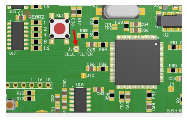
J1 (Cell Filter) solder jumper should be closed as well, using solder.
