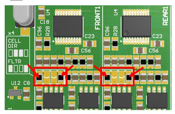
Within each red box, there are 4 solder jumpers. To ENABLE the filter, a solder connection should be made on the indicated positions (1 & 4). The other solder jumper should be left open (2 & 3) (image above)
