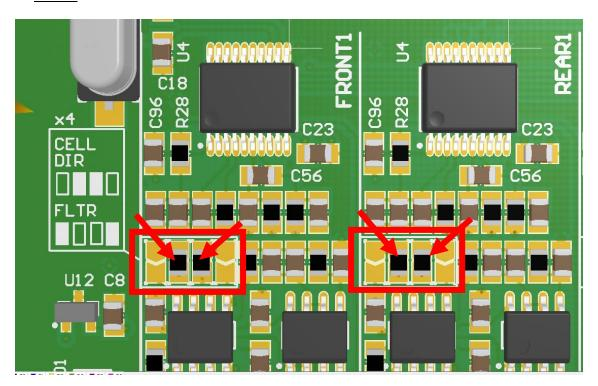
Within each red box, there are 4 solder jumpers. To ENABLE the filter, a solder connection should be made on the indicated positions (2 & 3). The other solder jumper should be left open (1 & 4) (image above)
