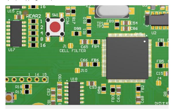
J1 (Cell Filter) solder jumper should be left open.
