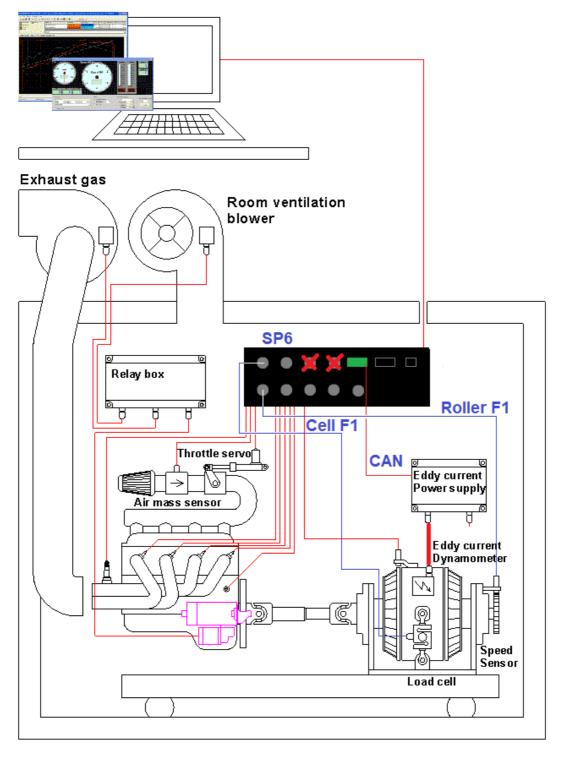
**Note**: SP6 can be installed close to the dyno / engine to shorten all data and control cables, and then only the serial cable will have to go through the wall to the computer. All control tasks will be performed
