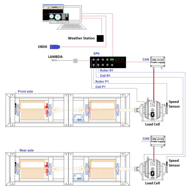
Note: **speed sensor** is recommended to be mounted at **brake side** to avoid the oscillations caused by the elastic couplers
