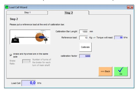
Note: if no calibration arm is available, **calibration can be performed directly over the cell** with the following considerations:
