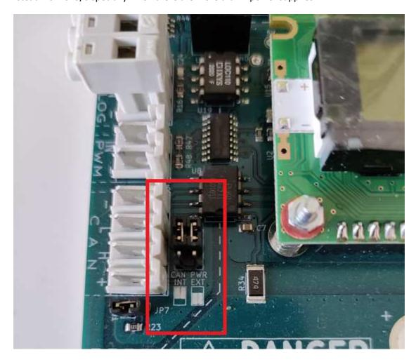
In the first **PWS3.3 units** (not PWS3.3b), the JP3 jumper should be set at the left side. And a small wire must exist between pins PWM- and GND- (it can be checked with a multimeter over those pins, without removing the PCB)
