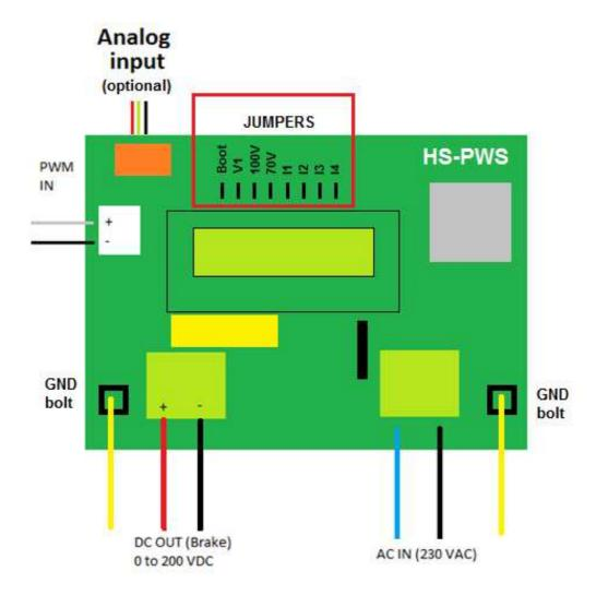
Note: **brake must not be operated without the GND wire**. If brake has leakages it must be repaired before using it with the Power Supply
