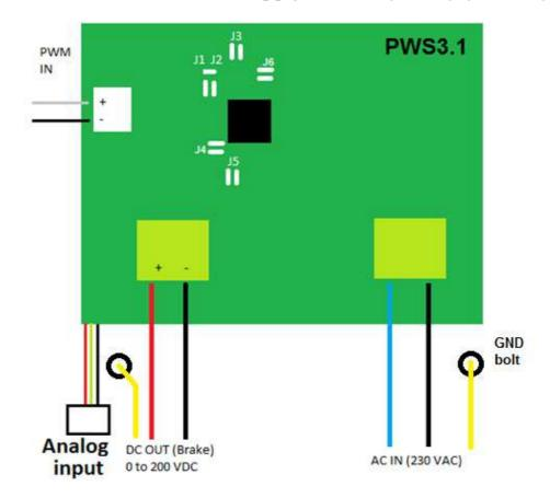
Note: **brake must not be operated without the GND wire**. If brake has leakages it must be repaired before using it with the Power Supply
